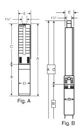
NOTES: All models suitable for use in 4" wells, unless otherwise noted. \* Built into sleeve 11/4" NPT discharge, 5" min. well dia.
