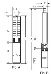
NOTES: All models suitable for use in 4" wells, unless otherwise noted. \* Built into sleeve 1½" NPT discharge, 6" min. well dia. \*\* Weights shown are in lbs. for pump end only.
