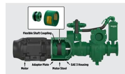
The Pioneer Pump® ElectricPAK™ uses a proprietary bracket design that rigidly connects the pump and motor together. The bracket, also known as a motor stool, is engineered to precise tolerances to ensure that the coupling remains aligned and protected.
